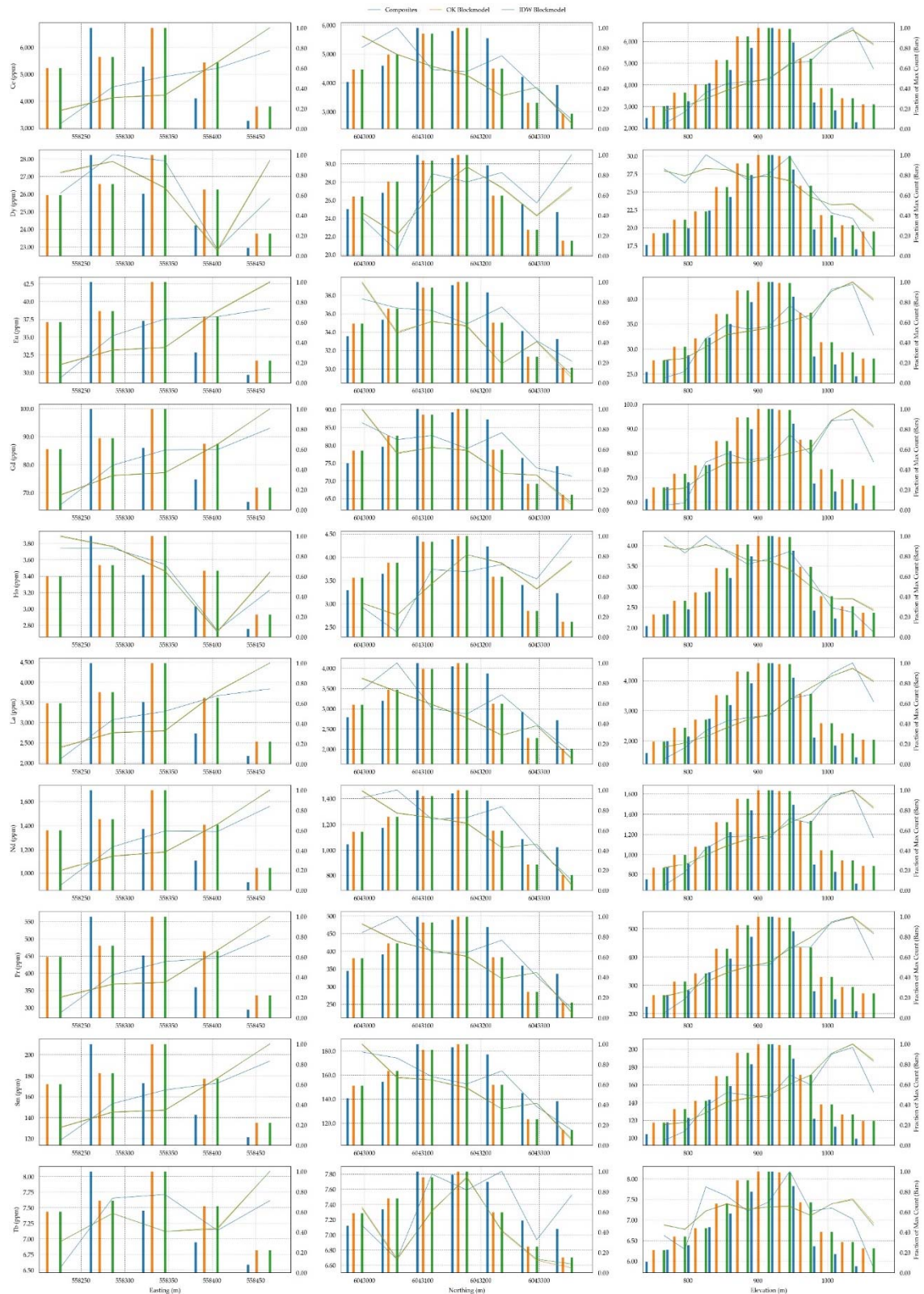
Figure 14.14. Swath plots of composite values versus estimated block model values in the Xenolithic Carbonatite.
